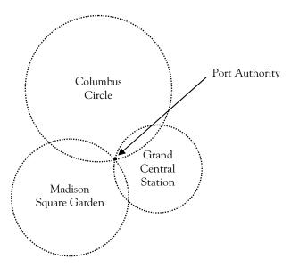
This process of calculating a single location using multiple linear measures is known as trilateration.<sup>34</sup> GPS receivers use trilateration in three dimensions (based upon information received from four satellites) to calculate their latitude, longitude, and altitude.<sup>35</sup> In addition, a receiver can compute its speed and the direction in which it is traveling by assessing the rate of change in information received from the satellites.<sup>36</sup>
